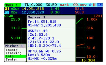
The *«Center»* menu option can be used to set the center frequency at the marker's frequency value.
