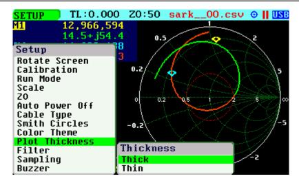
The screenshots below show graphs with plot thicknesses set to "Thick" and "Thin":
