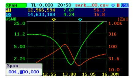
(ii) Use Navigator A to select **«SPAN»** in the main menu. Then use Navigator B to change the span. The span will change according to the current span frequency multiplier. The span frequency multiplier can be changed from the popup dialog, see (i) above.
