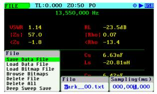
The analyzer stores the measured data at the specified interval. Number #n in the status line indicates the current record index
