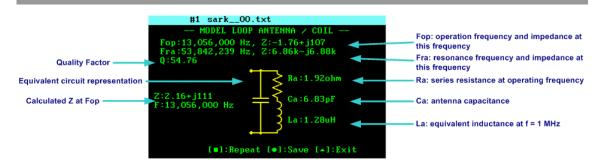
The internal procedure performed by the analyzer is as follows: the analyzer measures the impedance at 1 MHz and at the desired operating frequency (e.g. 13.56 MHz). Then it searches for the antenna's self-resonant frequency and measures the impedance at that point. The following parameters are extracted from these measurements:
