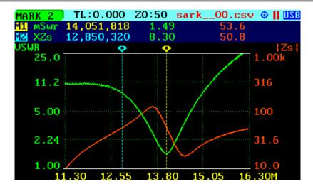
The *«Info»* option displays detailed information of the readings at the marker position, including the difference in frequency between both markers. One possible use of this feature is determining the VSWR bandwidth of an antenna.
