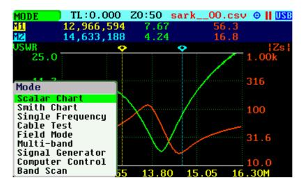
Use Navigator B to highlight the desired submenu mode option. Press the Select [■] button to validate the selection. Press any other button to cancel the operation.
