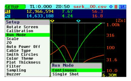
In continuous mode the analyzer is constantly sweeping provided that it is not in on hold state. In single-shot mode the sweep automatically stops on completion. Press the Run/Hold [>||] button to start a new sweep. Notice that in the stop condition the power consumption is reduced, so using single-shot mode helps to increase the battery autonomy.
