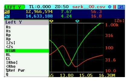
(ii) Use Navigator B when either the «LEFT Y» or «RIGHT Y» option is highlighted. Options are selected sequentially.
