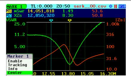
Since firmware version v0.10.6, there is the new *«Data»* menu option that allows selecting the data to the display at the marker position.
