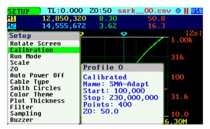
Once the calibration profile has been selected, choose **«SETUP»** *«Calibration» «OSL»* to start the OSL calibration procedure.
