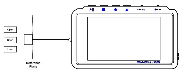
The analyzer performs a series of measurements with these loads, calculating error coefficients that are stored in a file that is automatically loaded each time the analyzer is run. These error coefficients are used to correct the measured values. The number of calibration points is fixed to 400.
