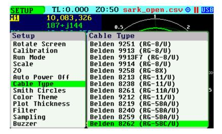
The transmission line length has to be entered into the **«TL LEN»** menu option within the Main menu. Use negative quantities for Subtract operations (transpose to load) and positive quantities for Add operations (transpose to input).
