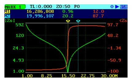
Select **«MARK 1»** *«Info»*. The readings show a length of 3.037m and a length difference (M1-M2) of 0.563m, which is the excess length of the piece of coax cable. Cut a piece slightly shorter than this value and repeat the process until getting to the expected value.
