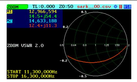
Since firmware version v0.10.9, the arrangement of the Smith chart mode changed slightly in order to display a bigger chart. Functionality and indicators have not changed.
