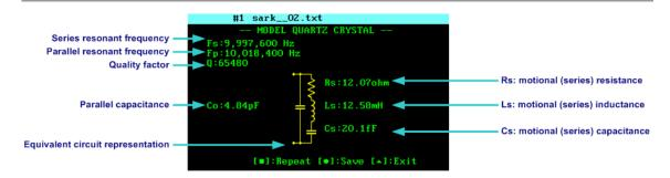
The process starts by searching for the series and parallel resonant frequencies. The start scan frequency is taken from the specified frequency value.
