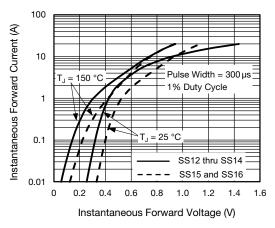
Fig. 3 - Typical Instantaneous Forward Characteristics
