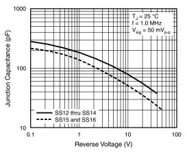
Fig. 5 - Typical Junction Capacitance
