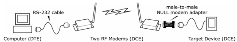
Figure B.3. Example of a MaxStream Radio Modem (DCE Device) connecting to another DCE device
