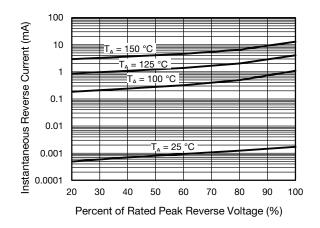
Fig. 4 - Typical Reverse Characteristics
