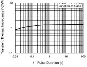
Fig. 6 - Typical Transient Thermal Impedance
