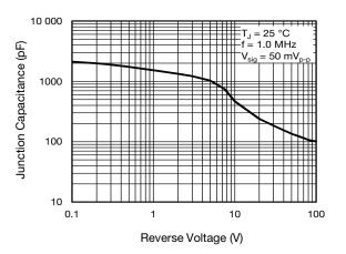
Fig. 5 - Typical Junction Capacitance
