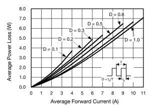
Fig. 2 - Forward Power Loss Characteristics
